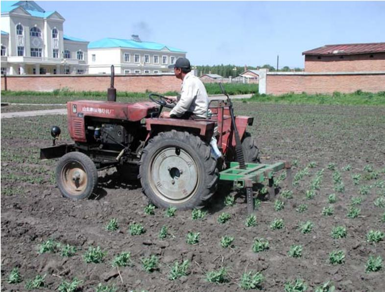
**The typical tractor we saw in Heilongjiang was powered by a one cylinder diesel engine mounted on two I-beams. In early June, they were being used to cultivate between the crop rows. Photos by Daryll E. Ray.**
